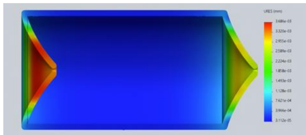
Figure 9. Version 2.0 of the lymphatic vessel: deformation test with open left valve and closed right valve (2020).
