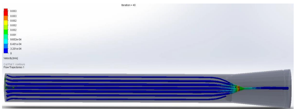
Figure 16. Computer velocity test simulation analysis of fluid with pressure of 32 mmHg to 25 mmHg (2020).
