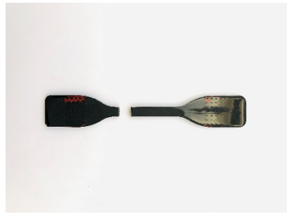
Figure 11. Fractured tension specimen.
