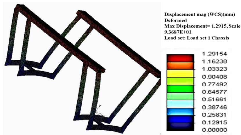
Fig. 13. Displacement analysis on Sub-frame assembly
