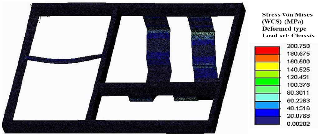
Fig. 8. Stress analysis on Chassis
