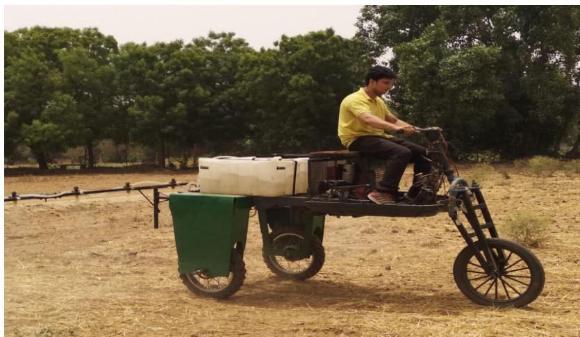
Fig. 15. Actual prototype of high clearance foliar applicator
