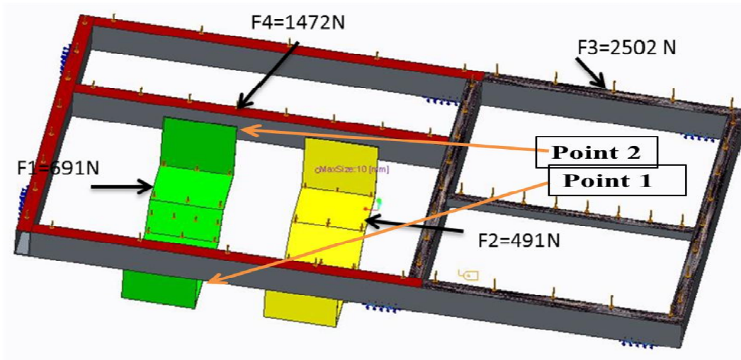
Fig. 6. Boundary conditions in Chassis
