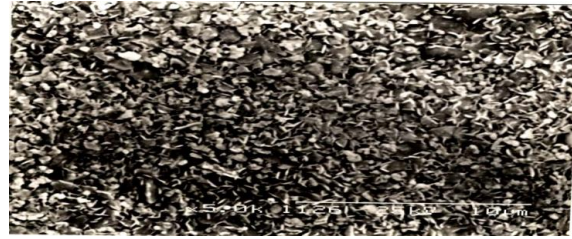
Fig. 2b. SEM micrograph of ZnO annealed at a temperature of 600°C for 2 hours
