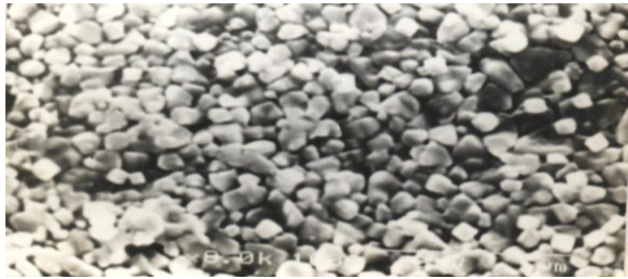
Fig. 2a. SEM micrograph of ZnO annealed at a temperature of 600°C for 1 hour
