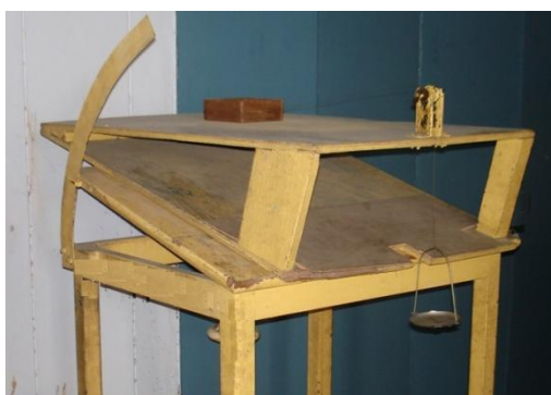
Fig. 3. Apparatus for measuring of static coefficient of friction
