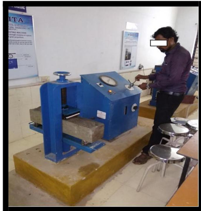
Image 1. The specimen testing of the flexural test in the laboratory
