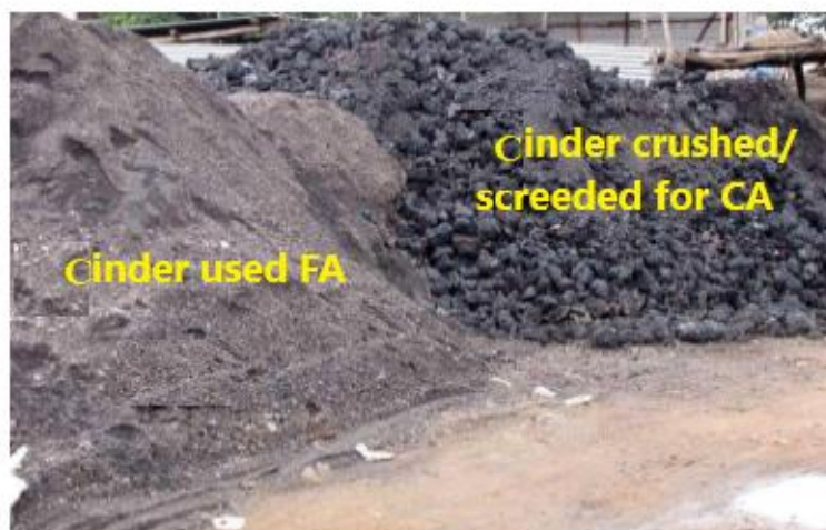
Fig. 1. Cinder from steel plants waste used as FA and CA for CC
