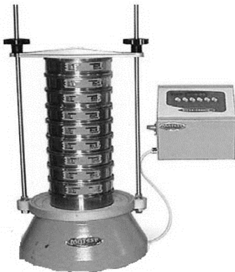
Fig. 1. Sieves arranged in a stack with the mesh size increasing from bottom to top on mechanical shaker
