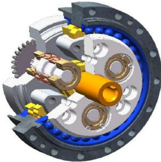
Fig. 1. Schematic diagram of RV reducer
