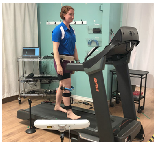
Figure 1. Knee kinematic acquisition system. Measures are captured while walking on a conventional treadmill.
