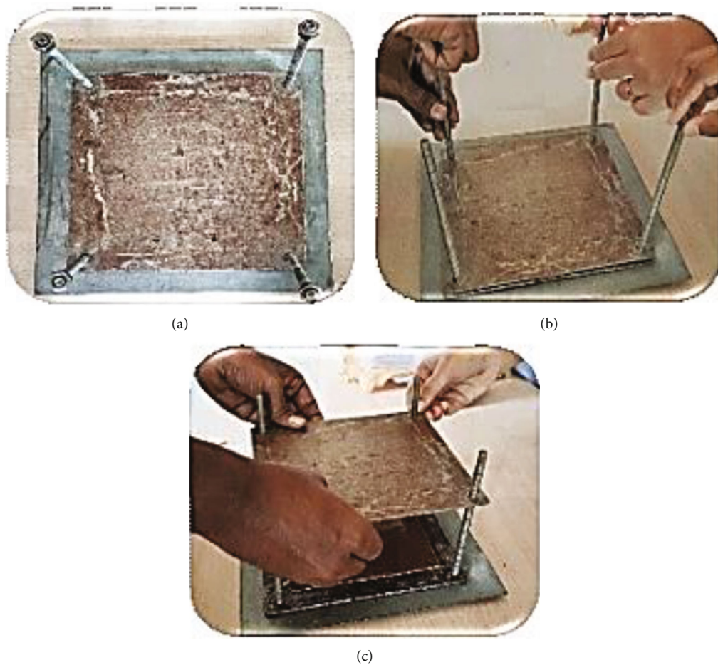
FIGURE 3: Fabrication of bio-based nanocomposites by using the hand layup method: (a) applying wax, (b) placing the woven mat, and (c) closing the mould.
